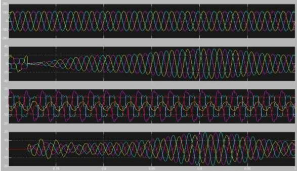
Fig 6. Simulation results: (a) Grid voltages, (b) Grid Currents (c) Unbalancedload currents, (d) InverterCurrents
