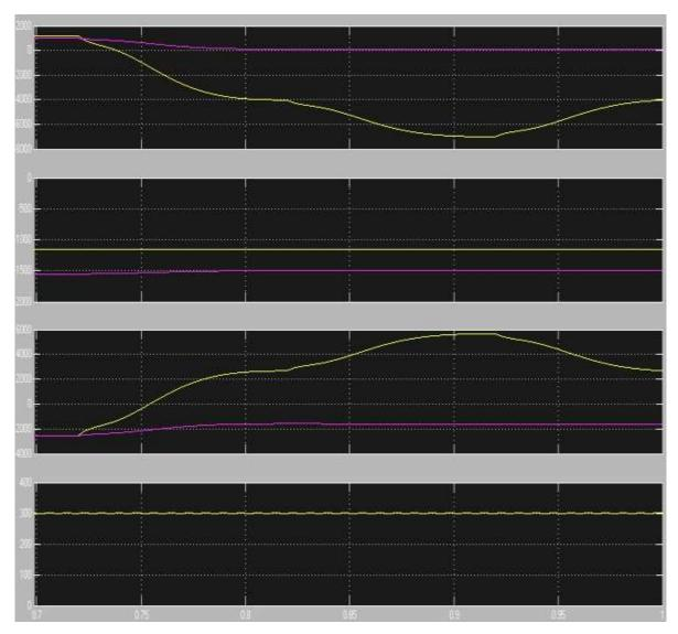
Fig 8. Simulation results: (a) PQ-Grid, (b) PQ-Load, (c) PQ-Inverter, (d) dc-link voltage.
