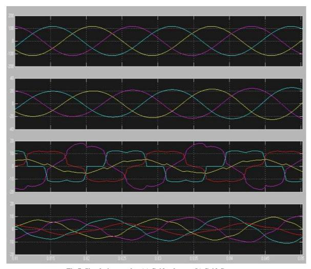
Fig 7. Simulation results: (a) Grid voltages, (b) Grid Currents (c) Unbalancedload currents, (d) InverterCurrents
