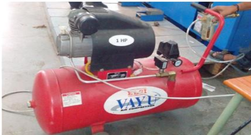
Fig. 3 Minimum Quantity Lubrication Setup with a Compressor
