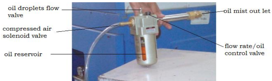
Fig. 2 Photographic view of MQL setup
