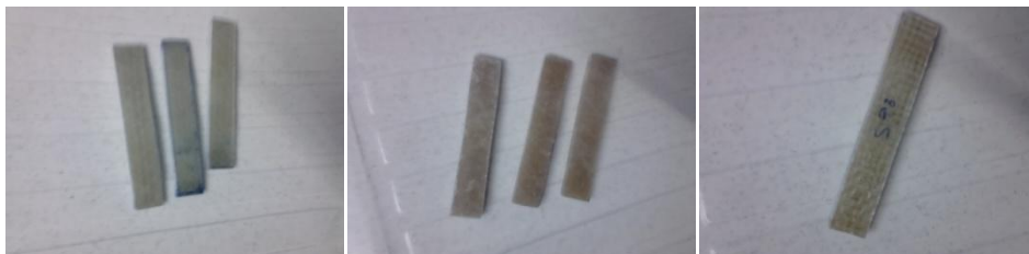
Fig 3.2: Flexural test specimens
