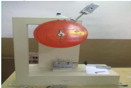
Fig 5.1: Izod Impact testing machine
