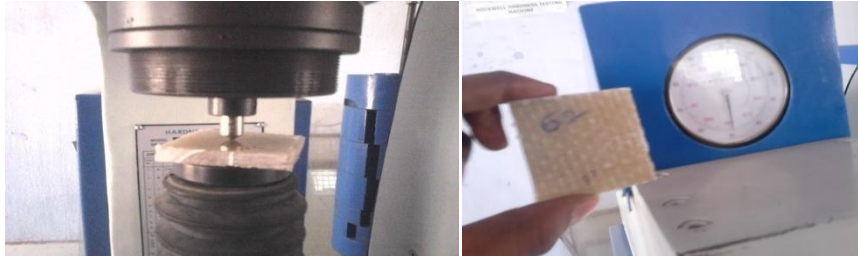
Fig 4.1: Hardness test Rig
