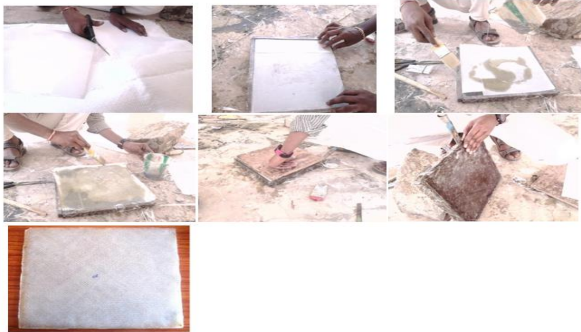
Fig 1.2: The preparation of Gfrp laminate
