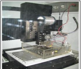
Figure1. WEDM experimental set up
