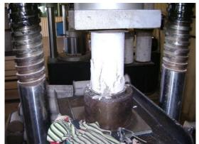
Fig. 2.1 Compressive Strength Test, conducted at the Laboratory of Building Materials Company Carlos Campos Consultoria and Construções Ltda. in Goiânia-GOIÁS
