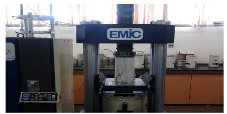
Fig. 2.2 Compressive Strength Test, conducted at the Laboratory of Concrete Department of Technical Support and Control of Furnas Centrais Elétricas S.A. in Goiânia-GOIÁS
