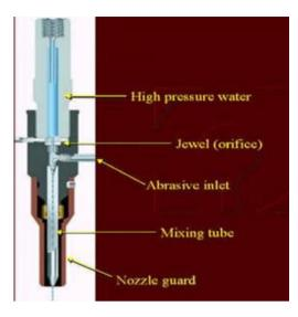
FIG: 3. Typical abrasive jet nozzle
