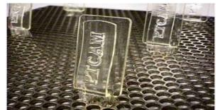
The platform at the end of a print run, shown here with several identical objects
