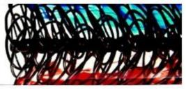
**SWIRL FLOW DEVICES:** Swirl flow devices causes swirl flow or secondary flow in the fluid .A variety of devices can be employed to cause this effect which includes tube inserts, altered tube flow arrangements, and duct geometry modifications
