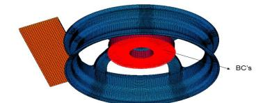
Figure 5. Boundary Conditions of Finite element model of the Wheel Assembly with Striker
