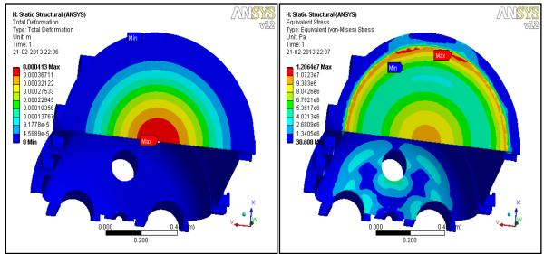
Fig 6.1 Max Deformation for the full body
