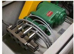
FIG: 2 Typical 20/30 horsepower crankshafts driven triplex pump.
