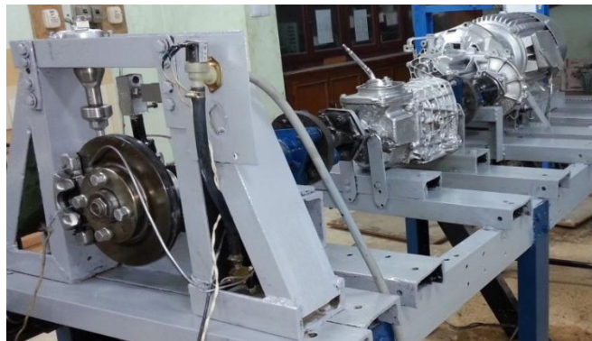
Fig. 1 Main components of the brake dynamometer.
