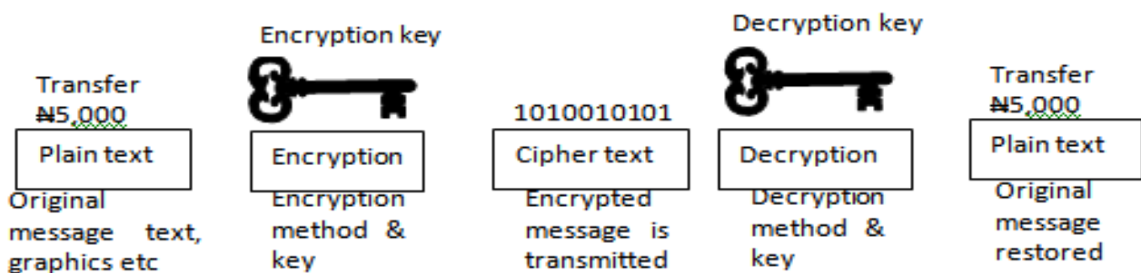
Figure 1: Symmetric key encryption
