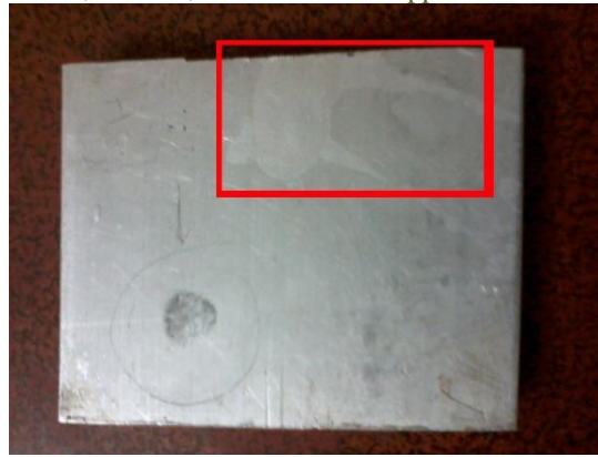
Fig 9 Red box denotes the area where reaction of NaOH on the Al metal has happened
