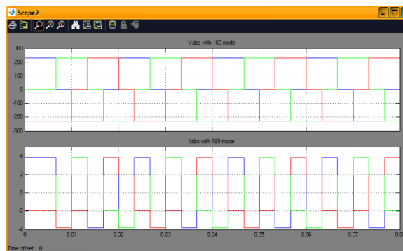
Fig.1.3. Three phase Load Current and Load Voltage waveform for inverter 180 0 mode of conduction without filter
