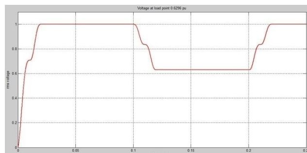
Figure4.1(a).voltage at load point is 0.6296 p.u TLG
