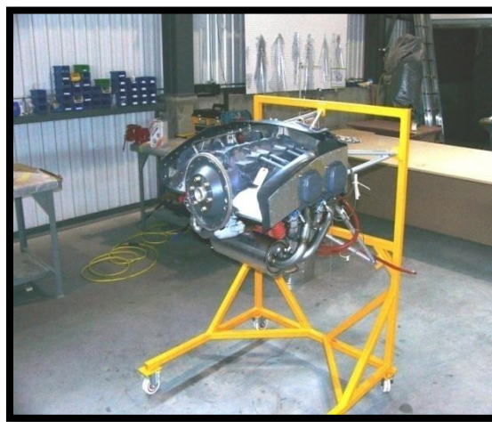
Fig. 8: Lycoming O-320-B Engine on Test Bed
