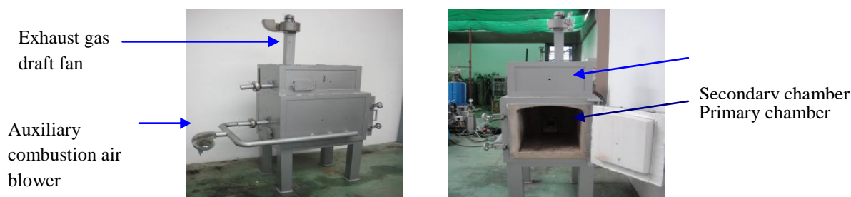
Fig.2 Prototype of double-chambered incinerator used in the experiment
