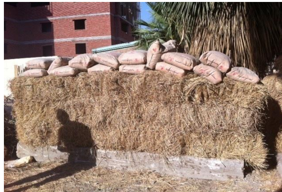
Figure 2: Pre-compression Test of full scale wall A
