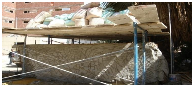
Figure 6: The loading technique on Wall B
