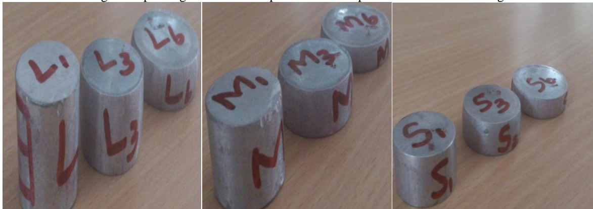
Fig.4. Deformed specimen for various aspect ratios -1.0, 0.8 and 0.6
