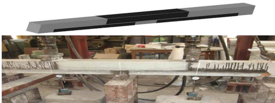
Figure 3.31 Strengthening pattern of SB8
