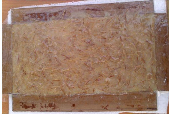
Fig 9: Mould Box with Un-Treated fibers and resin mixture
