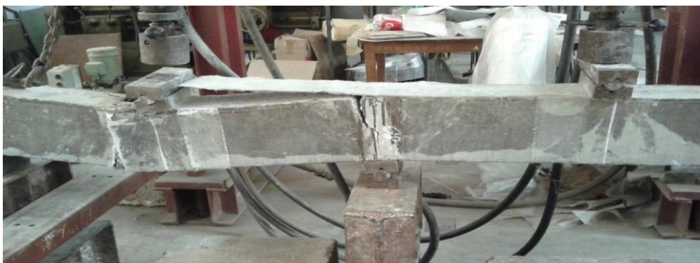
Figure 3.23 Failure of the beam by tensile rupture
