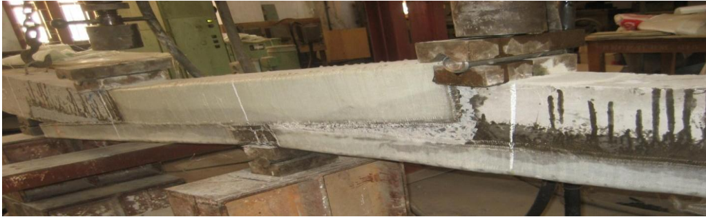
Figure 3.32 Failure of SB8 by debonding of GFRP
