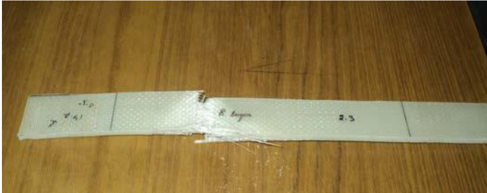
Figure 3.10 Specimen failure after tensile test
