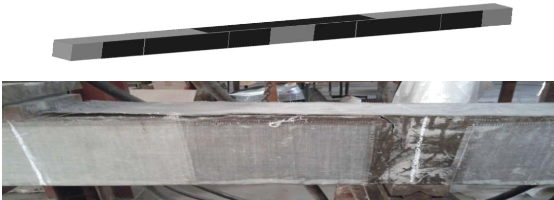
Figure 3.26 Debonding of FRP and cracking pattern above central support of the beam
