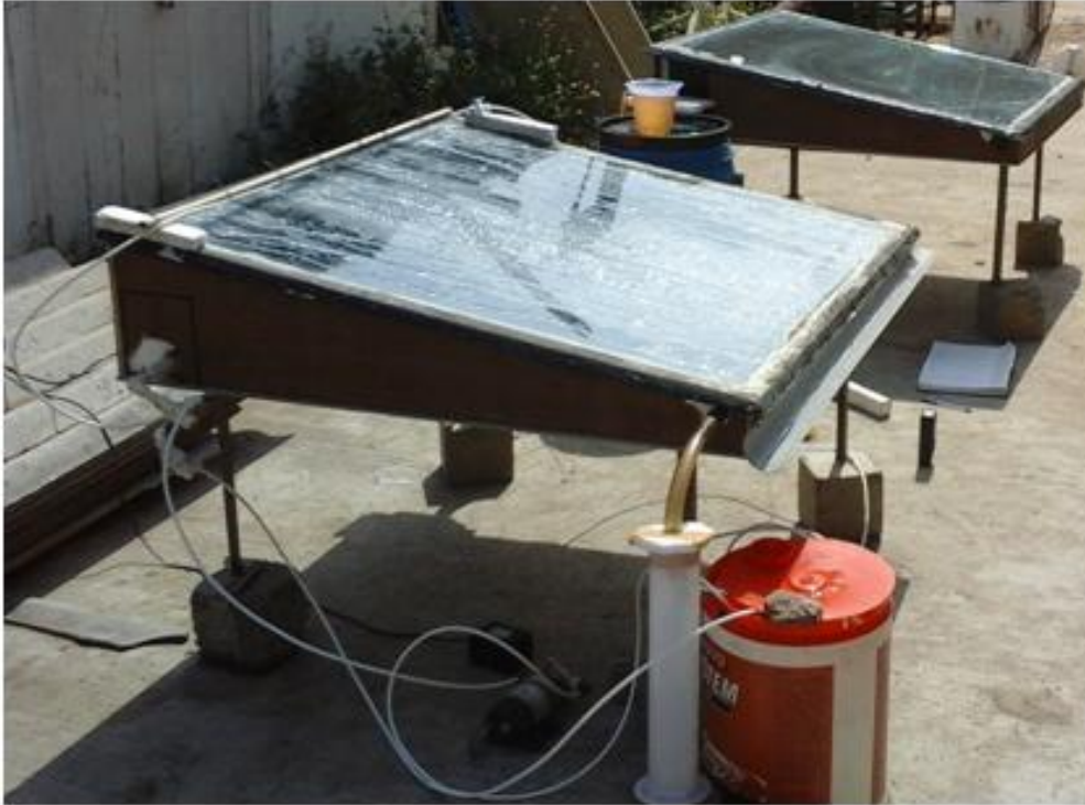
Figure 1: Experiment scheme for solar passive regenerator, with and without glass cooling
