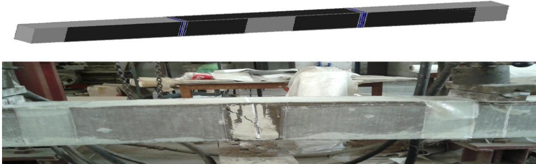
Figure 3.24 Cracking pattern at lower load value
