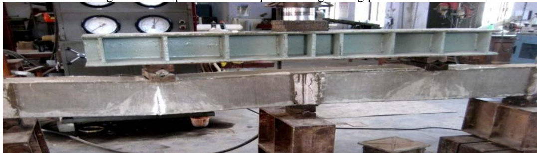
Figure 3.39 Failure of the beam by tensile rupture
