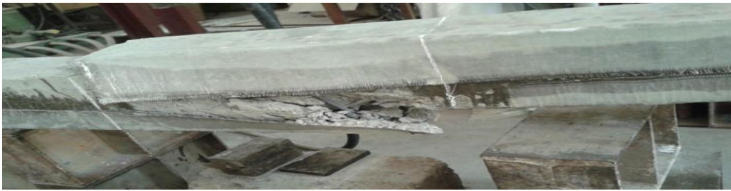
Figure 3.29 Shear crack in the left span
