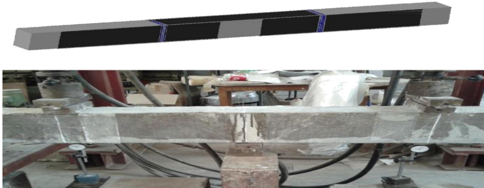
Figure 3.21 Strengthening pattern of beam SB4
