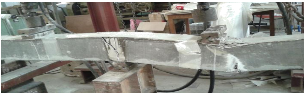
Figure 3.25 Rupture of GFRP sheet at mid section of the right span
