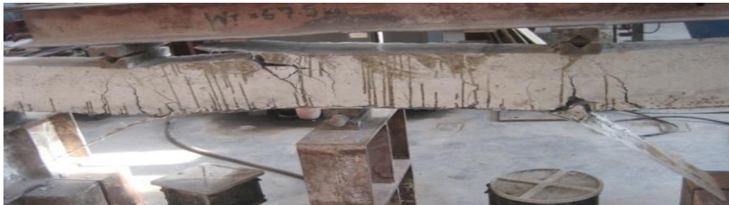
Figure 3.37 FRP sheet separations without concrete
