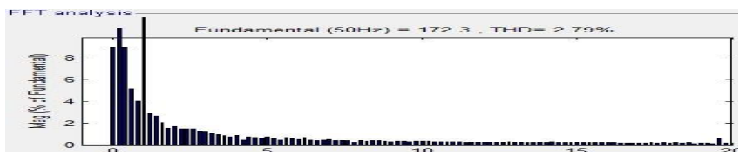
Fig 19: Current harmonics before transformer for Connection C
