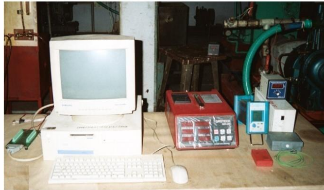
Figure.3. Photographic view of pressure and emissions measuring setup
