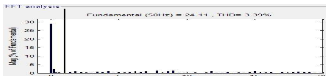
Fig 15: Current harmonics after transformer for Connection B
