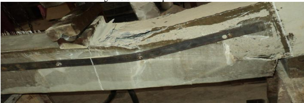
Figure 3.35 Magnified view of Debonding
