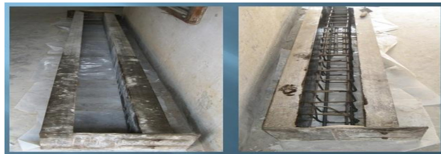
Figure 3.3 Steel Frame Used For Casting of Beam
