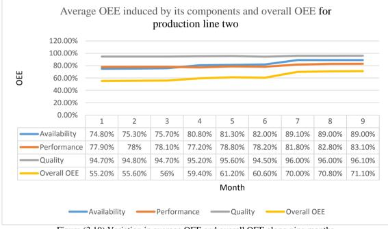
Figure (3.10) Variation in average OEE and overall OEE along nine months for production line two.
