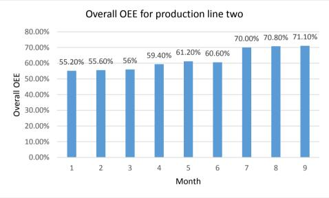
Fig (3.8) Monthly overall OEE for production line two along nine months
