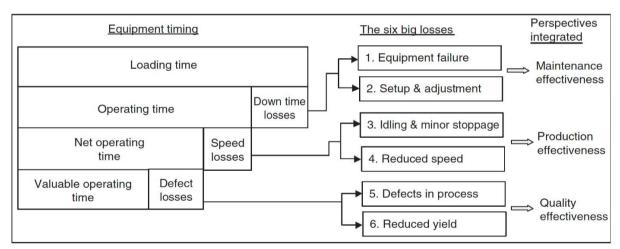
Figure (1.1) OEE measurement tool and the perspectives of performance integrated into the tool [10].
