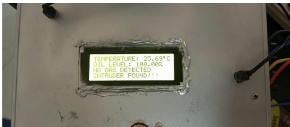
Figure 9: Intrusion Detection showing on the LCD
