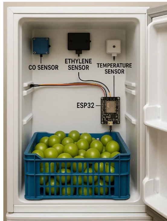
Figure 4.1: Implemented IoT Based Tomato Monitoring System
