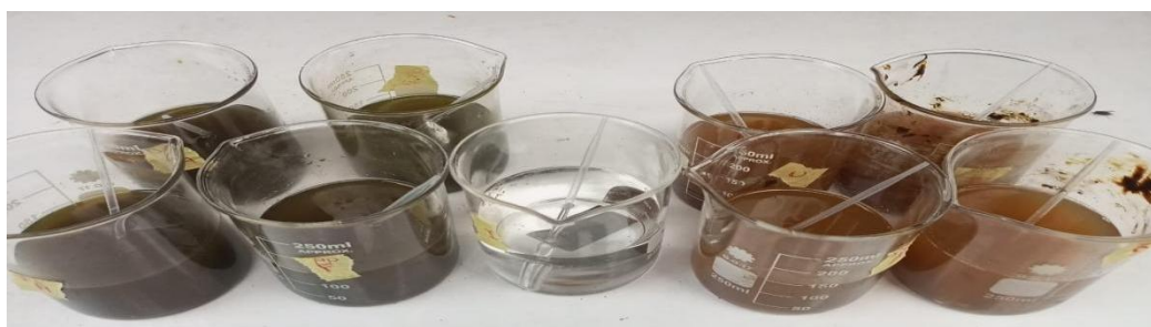
Figure 2: Pictures of Beakers to carryout Corrosion Experiments (Starting with Paw-Paw Extracts as Inhibitor, without Inhibitor, and finally Guava Extracts as Inhibitor)
