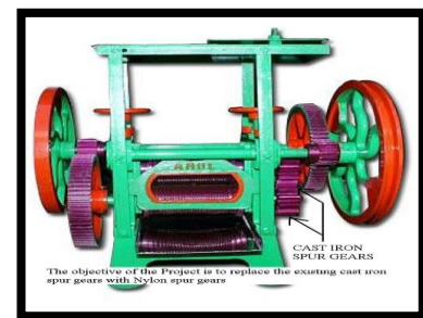
Fig. No. 1 Schematic diagram of a sugarcane juice machine.
