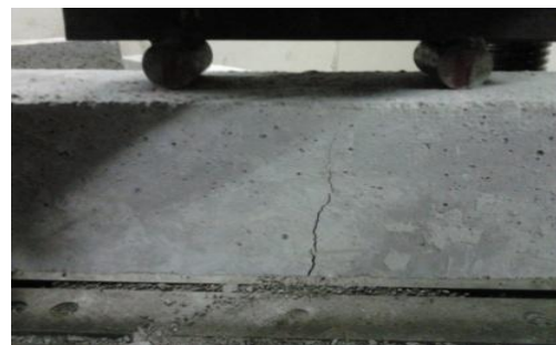
Fig. 2: Typical Beam Specimen Showing Crack at Failure
