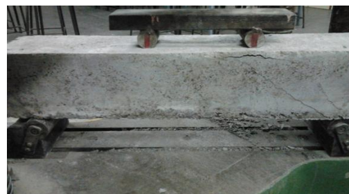
Fig. 3: Typical Beam Specimen Showing Shear Crack at Failure
