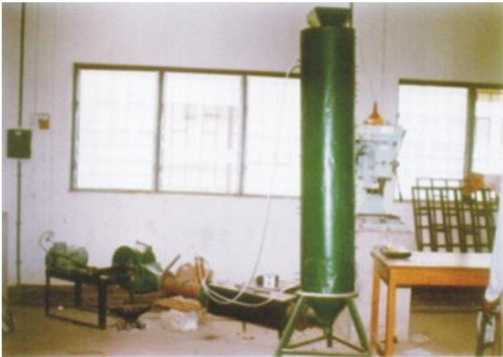
Figure 1: Experimental set up of fluidized bed dryer model plant
