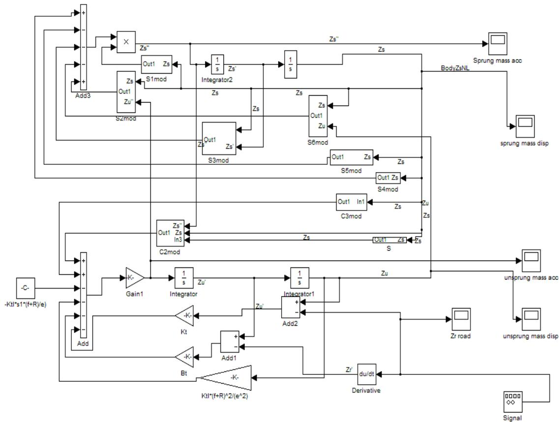
Fig.3.4: Simulink Block Diagram of Suspension System.
