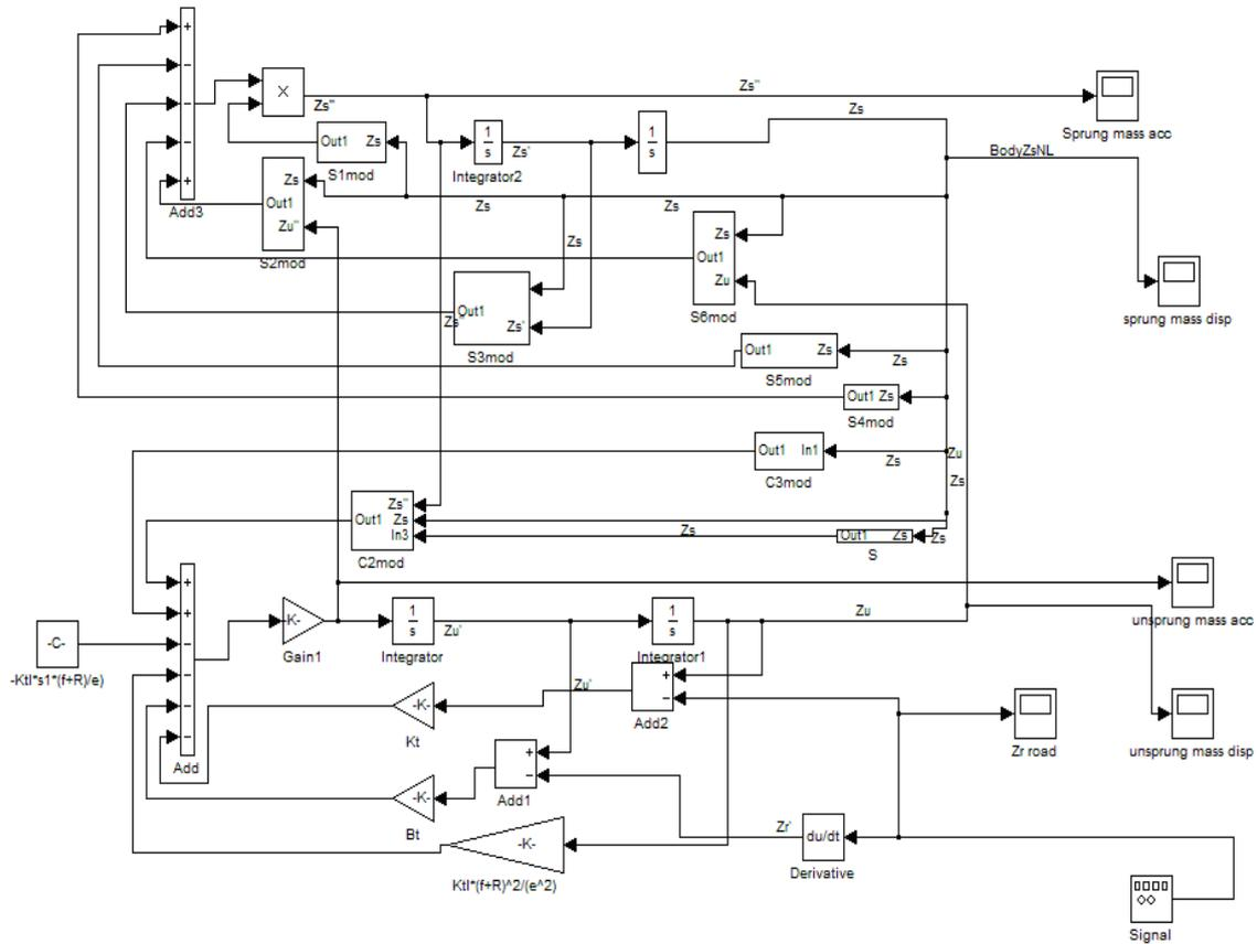
Fig.3.4: Simulink Block Diagram of Suspension System.
