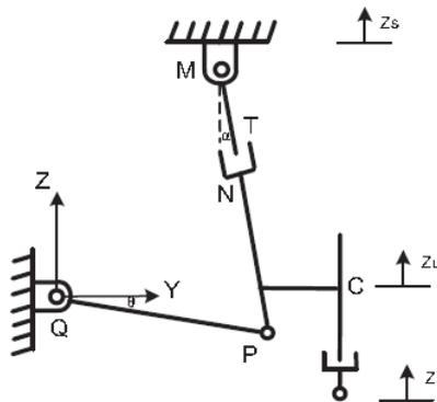
Fig.3.1:Kinematic model of MacPherson suspension
