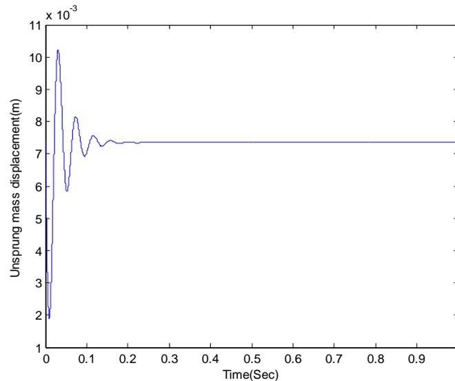
Fig.3.5: Displacement response of Chassis
