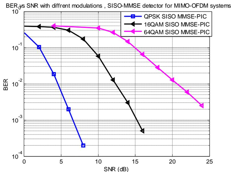
Fig. 7. BER vs. SNR performance of MIMO-OFDM systems based SISO MMSE-PIC detector with QPSK, 16QAM and 64QAM modulation
