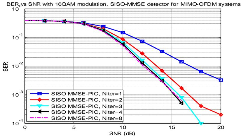
Fig. 3. BER vs. SNR performance of MIMO-OFDM systems based SISO MMSE-PIC detector with 16QAM modulation scheme and various iterations. The BCJR decoder is used.
