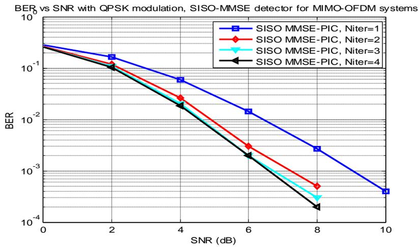
Fig. 4. BER vs. SNR performance of MIMO-OFDM systems based SISO MMSE-PIC detector with QPSK modulation scheme and 4x4 number of antennas.
