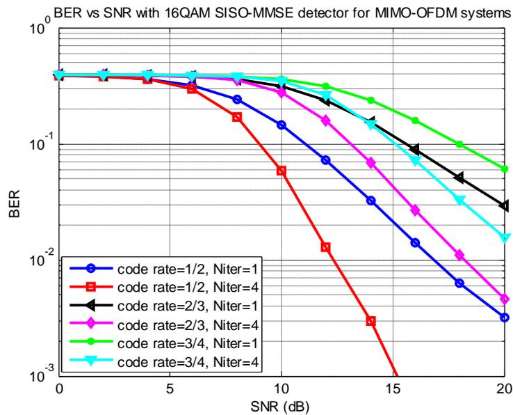
Fig. 6. BER vs. SNR performance of MIMO-OFDM systems based SISO MMSE-PIC detector with 16QAM modulation scheme and various coding rate 1/2, 2/3 and 3/4.
