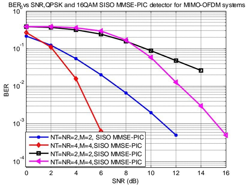
Fig. 8. BER vs. SNR performance of MIMO-OFDM systems based SISO MMSE-PIC detector for  $N_T = N_R = 2$  and  $N_T = N_R = 4$  number of
