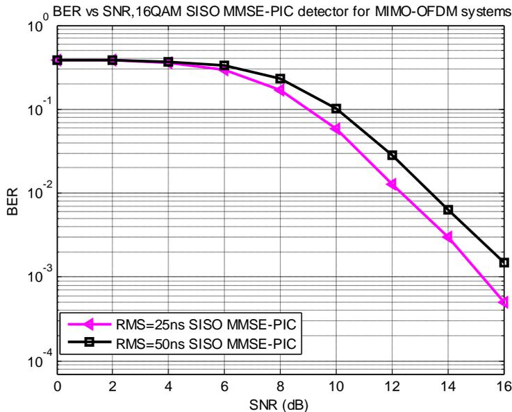
Fig. 9. BER vs. SNR performance of MIMO-OFDM systems based SISO MMSE-PIC detector for two RMS delay spreads 25ns and 50ns.
