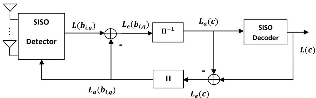
Fig. 2. MIMO iterative receiver scheme
