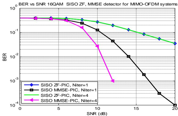
Fig. 5. BER vs. SNR performance comparison of MIMO-OFDM systems based ZF and SISO MMSE-PIC detectors with 16QAM modulation scheme and various iterations. The BCJR decoder is used.
