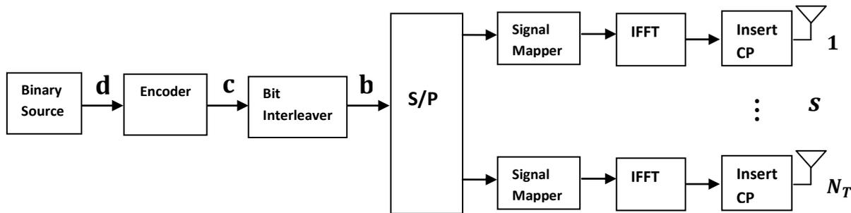
Fig. 1. Block diagram of MIMO OFDM transmission
