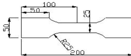
Fig. 2: Specimen for tensile test (all dimensions in mm).
