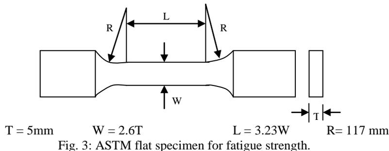
Fig. 3: ASTM flat specimen for fatigue strength.
