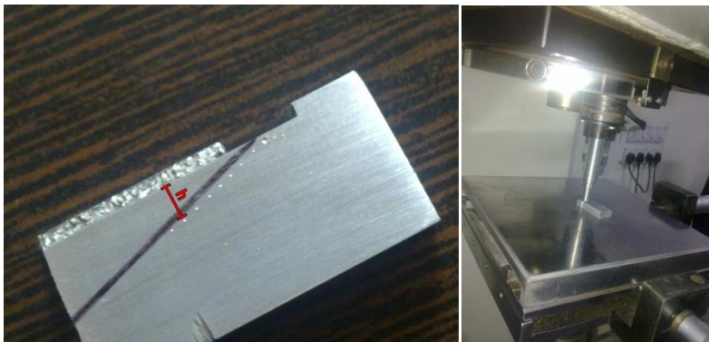
Fig 12 (Left) The cross section area where indentation was made to measure the hardness. (Right) Vickers Hardness tester
