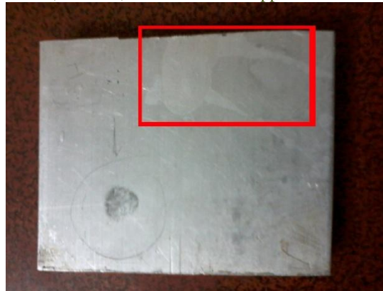
Fig 9 Red box denotes the area where reaction of NaOH on the Al metal has happened
