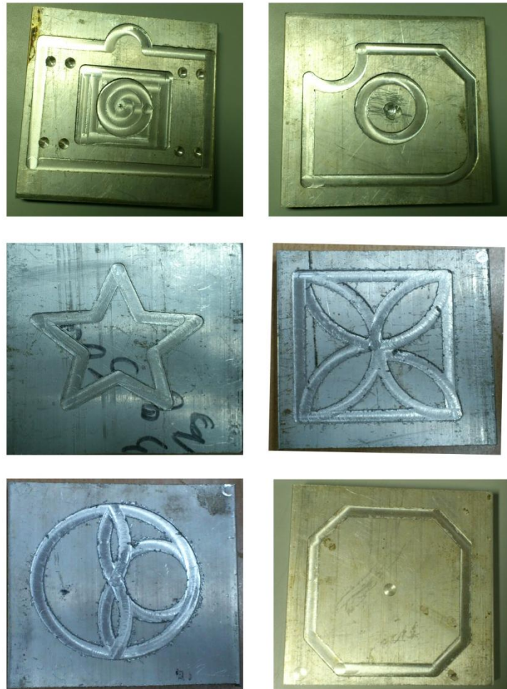
Fig 4 Various lines and curves done using the 3 DOF CNC milling
