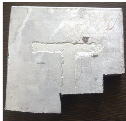
Fig 11 The chemically etched test specimen (the formation of the T structure)
