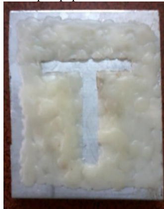
Fig 10 Wax applied as a maskant on the Al test specimen
