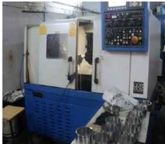
Fig 4.4 CNC Turning Centre
