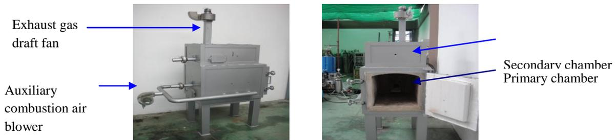
Fig.2 Prototype of double-chambered incinerator used in the experiment
