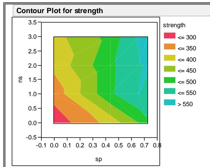
Figure 6: Contour plot correlating NS and SP with compressive strength actual results.
