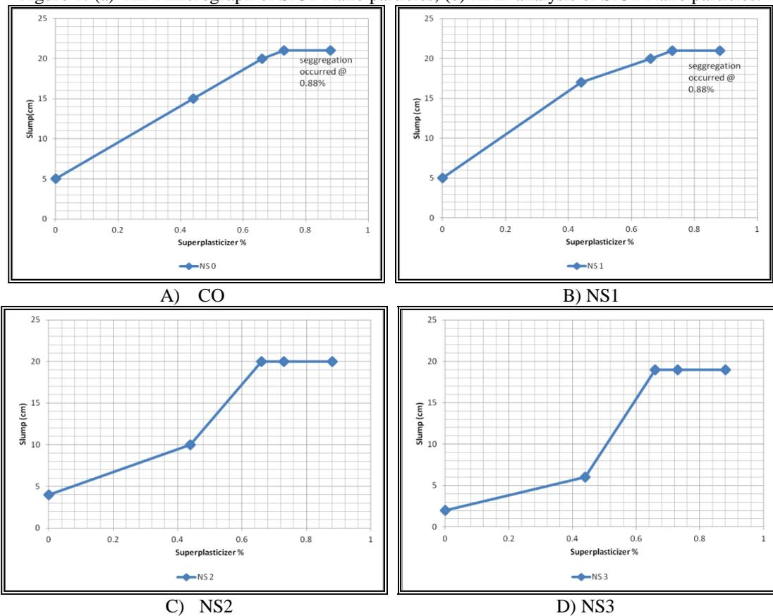
Figure 2: Effect of increasing SP on the slump of different NS concrete.
