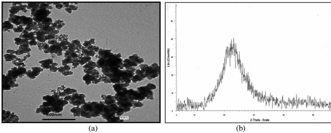
Figure 1: (a) TEM micrograph of SiO<sub>2</sub> Nano particles, (b) XRD analysis of SiO<sub>2</sub> Nano particles.
