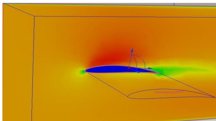
Figure 2: computation Analysis of NACA 65420
