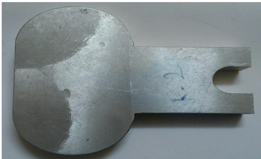
Fig. 17. casting with feeder of diameter 50mm and sleeve thickness 10mm shows no defects after machining
