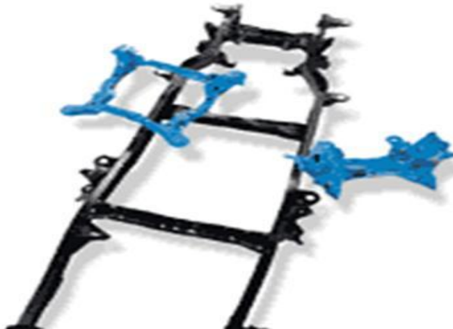
Fig. 10 Automobile components (frames) produced by MPW process (Source: Dana Corporation, USA)
