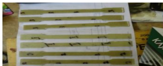
SPECIMANS FOR TENSILE TEST ASTM D638
