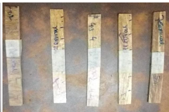
Fig: 8 Flexural test specimens after fracture.
