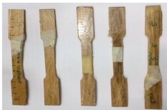
Fig: 7 Tensile test specimens after fracture.
