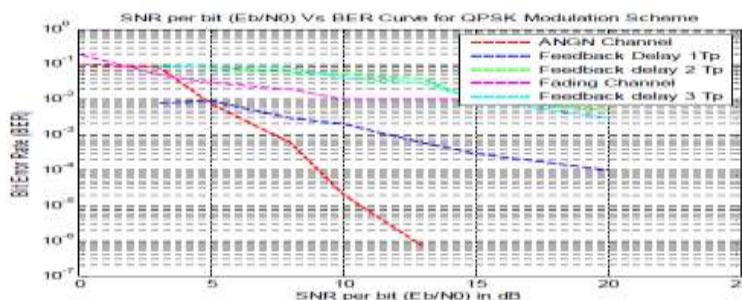
Figure 2 Performance at Step size =1dB, Fading Rate =50Hz
