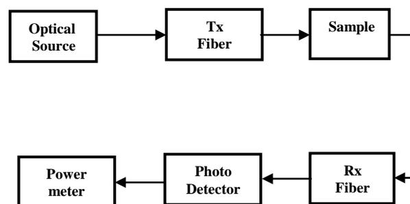
Figure 1 Block diagram of the measurement setup.
