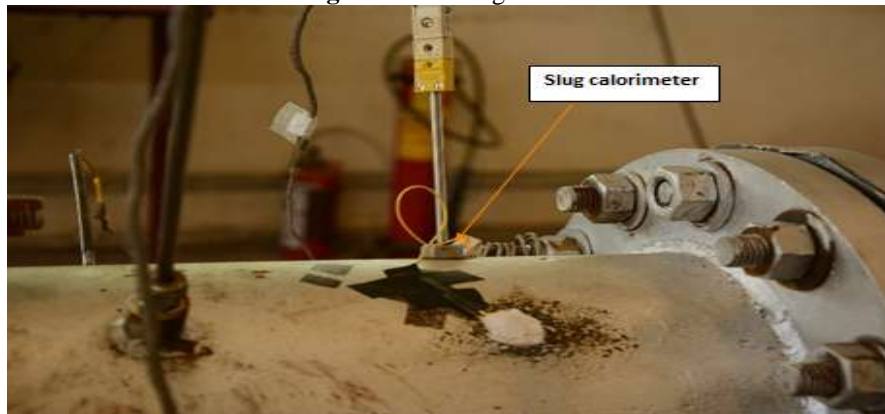
Figure 3: Copper Slug Calorimeter Mounting
