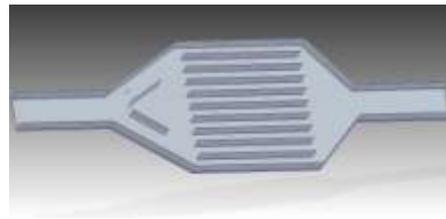
Fig 1.2: Heat sink with rectangular channels and diverter
