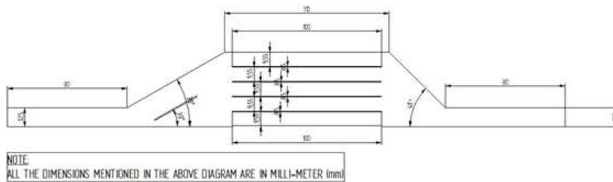
**Fig 2.2:** Heat sink with diverter
