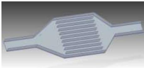
Fig 1.1: Heat sink with rectangular channels
