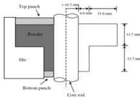
Fig. 4. Geometry and boundary conditions of a rotational flanged component.
