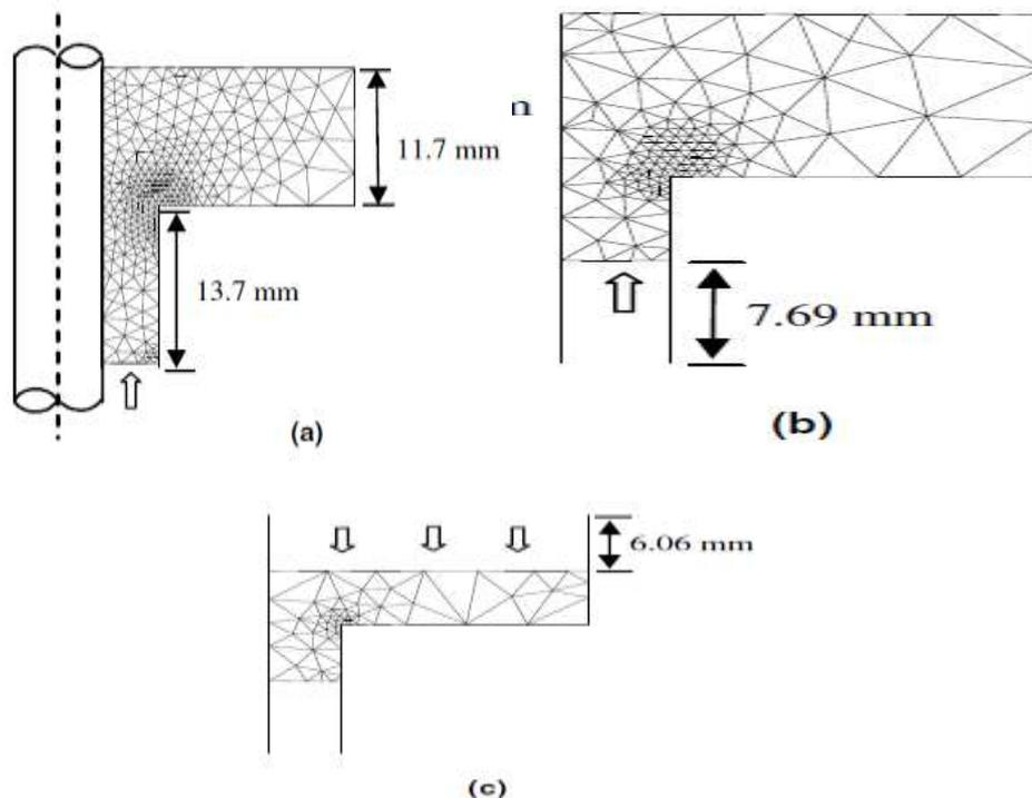
Figure Axisymmetric representation of compaction process with tool path and position during compaction process. (a) Step begins, (b) end of step and (c) end of final step
