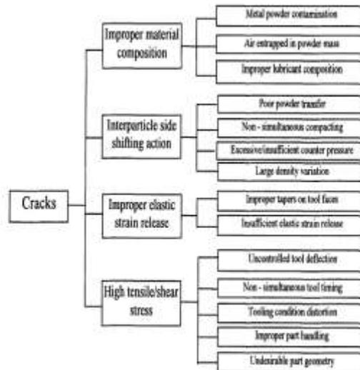
Figure 1. General causes of cracks in green P/M compacts and some example conditions.
