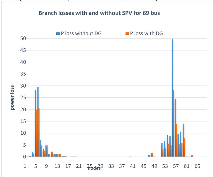
**Fig 2.** Branch active losses without and with SPV for 69-bus.
