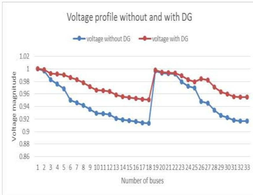
Figure 4. The voltage profile of 33-bus without and with DG integrated.
