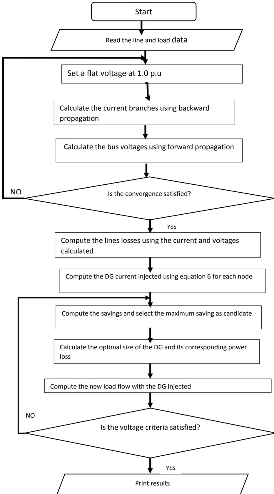
Fig1. Flowchart of BFSM for optimal DG placement
