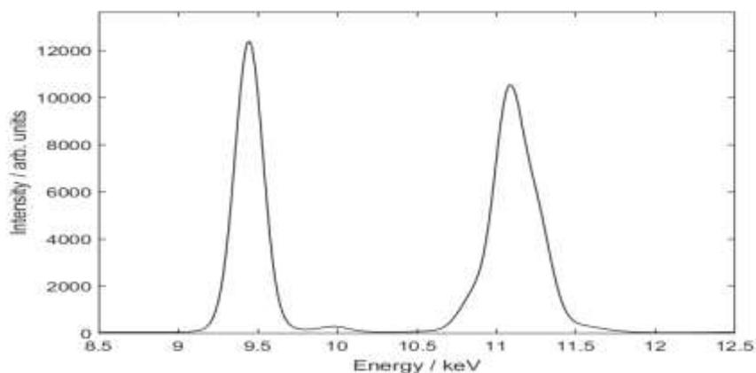
**Figure 3:** Region of the XRF spectrum containing the most intense Pt peaks. This spectrum is taken from a pure (>99.99%) platinum foil.
