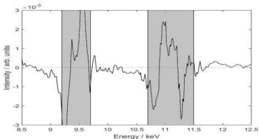
**Figure 6:** To check that there are no mercury peaks present in the reference platinum sample we show here subtracted spectra for two areas of the platinum reference foil. No mercury peaks are visible. As with the previous figure, the energy regions containing the strong platinum peaks are shaded to indicate that we would expect small changes in instrument energy scale and sensitivity to make these areas noisy and unreliable.
