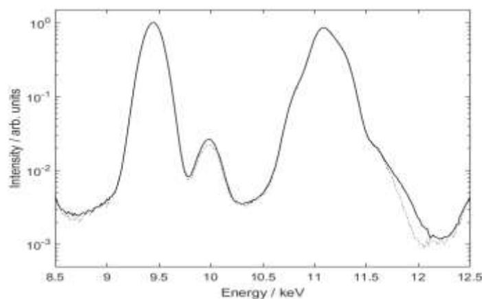
**Figure 4:** Semilogarithmic plot comparing XRF spectra from a pure platinum surface (stippled line) with a 20.5 $\mu$ g/cm<sup>2</sup> mercury reference material placed on top of this pure platinum sample. The main differences in XRF intensity are around 10keV and just below 12keV, where the most intense mercury lines occur. However the difference in intensity is small compared to the large, intense platinum peaks.
