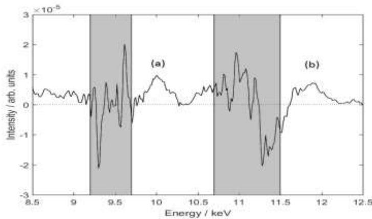
**Figure 7:** Spectrum from the Royal Society platinum Troy pound, with the spectrum of the pure platinum reference foil subtracted. Shaded areas are unreliable (for the same reason as in the above figures). Mercury x-ray peaks (a) and (b) are clearly visible. These mercury peaks are the  $L_{\alpha 1}$  and  $L_{\beta 1}$  Hg x-ray lines at 9.99keV and 11.82keV respectively.
