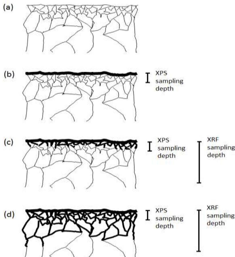
**Figure 1** Schematic cross-section of a polished prototype kilogram, (a) immediately after manufacture, (b) Some tens of days after manufacture, (c) about 10 years after manufacture and (d) about 100 years after manufacture. Darker lines represent a high mercury concentration. XRF is able to capture mercury signal from a much deeper region than XPS. This diagram is schematic: in reality the XRF sampling depth is around 2,000 times larger than the XPS sampling depth.
