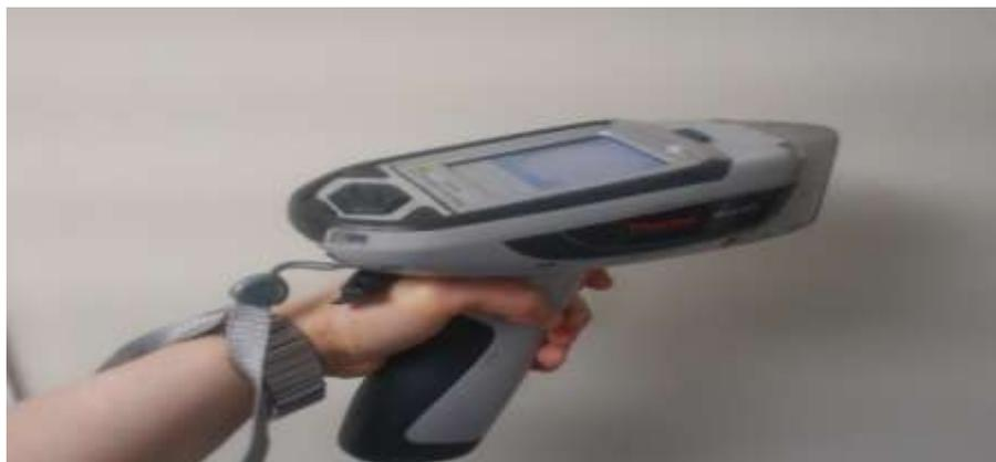
**Figure 2** Handheld, energy-dispersive X-ray fluorescence (XRF) instrument used in this work. It operates in air, and requires no vacuum. It is a non-destructive and non-contact chemical-element analysis instrument.
