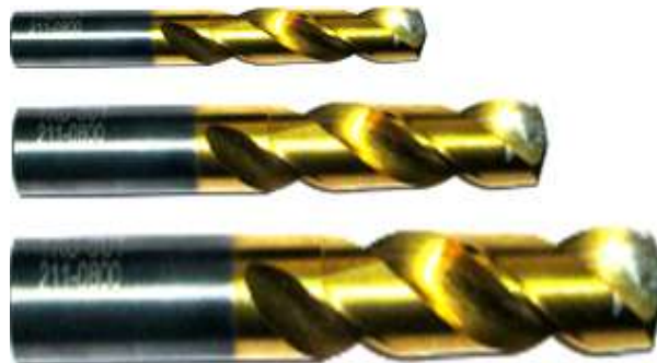
Fig.2 TiN coated solid carbide twist drill bits used for experiments
