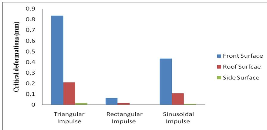
Fig. 15: Effect of triangular, rectangular and sinusoidal impulsive force on different surfaces of the building
