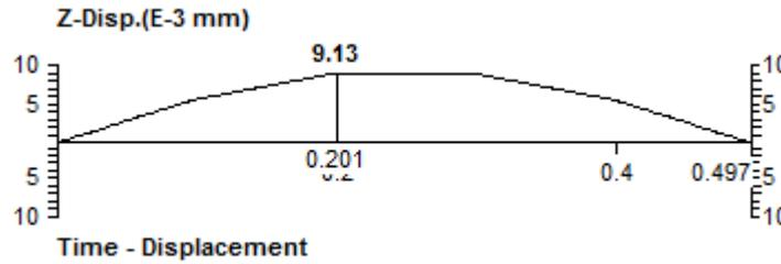
Fig. 14: Critical deformation on side surface of the buidng
