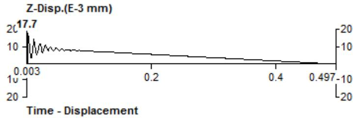
Fig. 6: Critical deformation on side surface of the building in Z-direction
