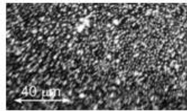
Fig. 2. Silicon carbide precipitates
