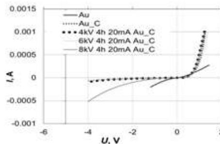
Fig. 4. Volt-Ampere characteristics of pn junctions
