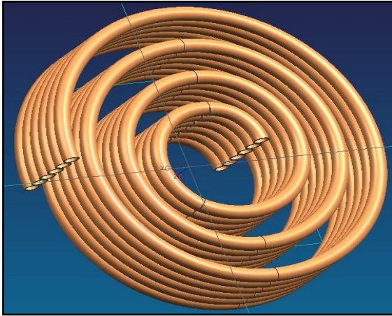
Fig. 5 Spiral tube bundle
