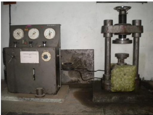
Figure3 compression testing machine (200t capacity)
