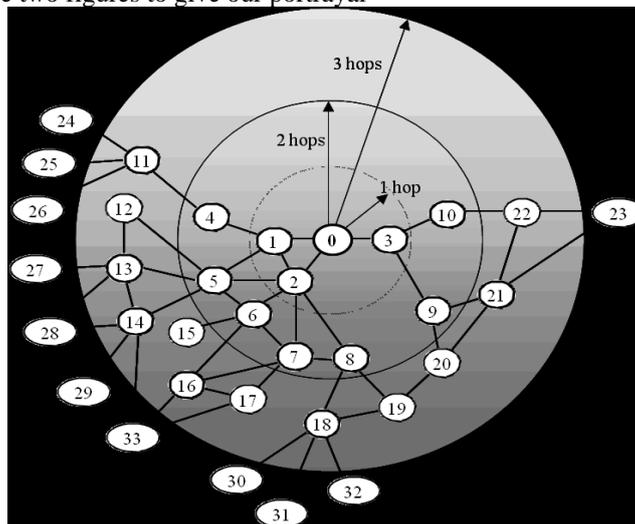
Fig. 3. System structure. Node 0 is a server node, and others are clients.
