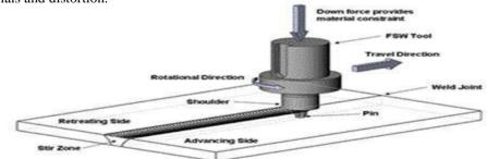
Figure 1 Schematic diagram of FSW Process
