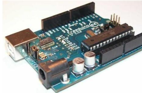
The Freeduino is an open source microcontroller board based on the ATmega8/168/328. It has 14 digital input/output pins (of which 6 can be used as PWM outputs), 6 analog inputs, a 16 MHz crystal oscillator, a USB connection, a power jack, an ICSP header, and a reset button. By plugging in a USB cable into the Freeduino, we can be able to upload the programs to the microcontroller. And also by providing the External adapter to the Freeduino, we can activate the Freeduino board.
