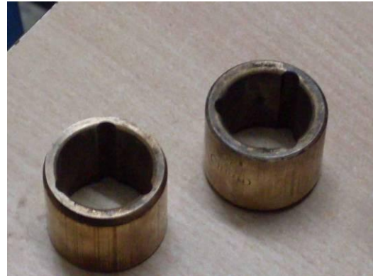
Figure 1.0 Worn out bearing bush (Courtesy VIRA PUMPS)
