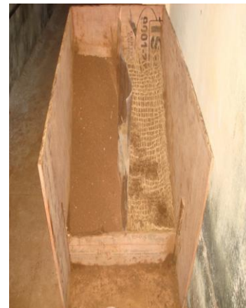
Figure. 6. Landslide model constructed in the laboratory
