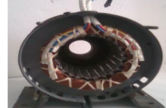
Fig. 2: Developed prototype of stator core of induction motor
