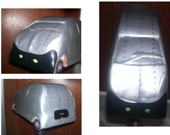
Fig. 2. Location of Base bleeds in car model
