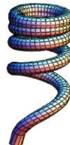
Figure 8. A tubular helical surface with a centerline of variable step
