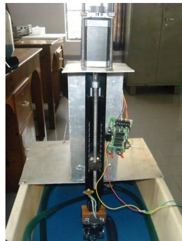
Fig. 2: Low cost Sinker EDM
