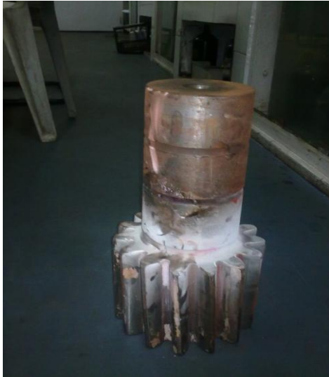
Figure3: Helical pinion of traction motor
