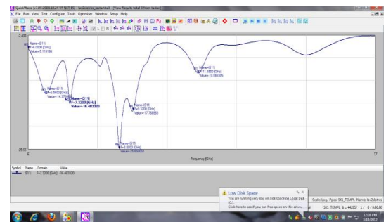
Fig15:Return loss of design with 2 U-slots and slot rotated to 90^\circ
