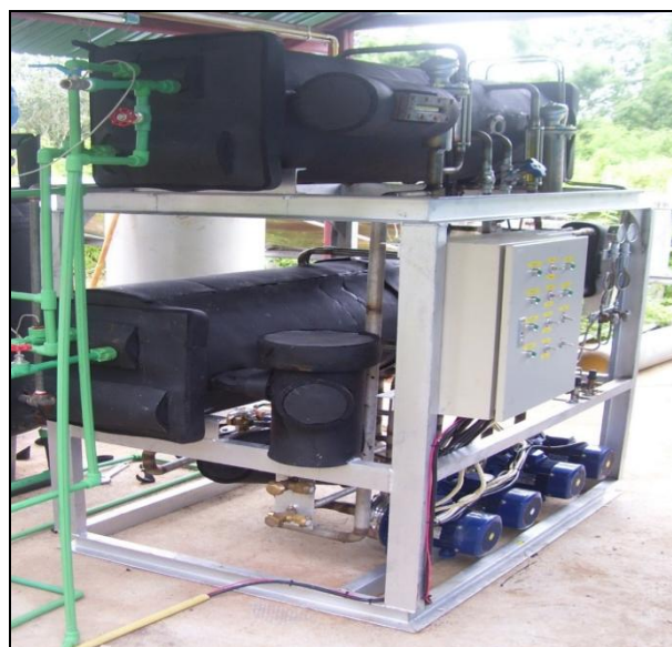
Figure 5. The prototype of absorption heat transformer.
