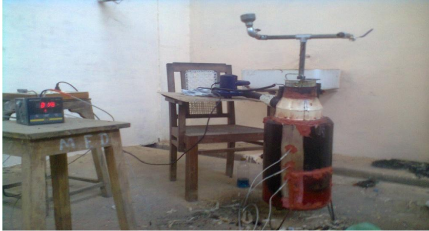
Fig.3.1- Experimental setup of updraft biomass gasifier
