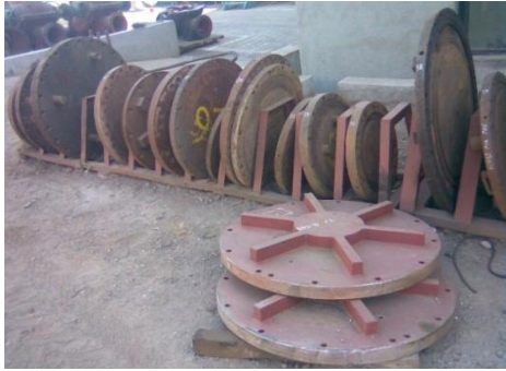
Photo 5.3: Situation of pressure plates before improvement
