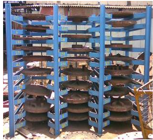
Photo 5.4: Improved situation of pressure plates
