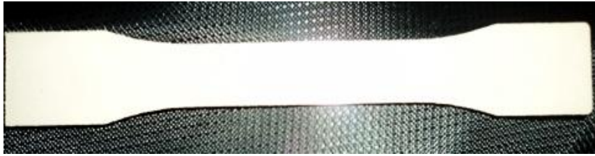
Fig: Tensile specimen As per ASTM D638
