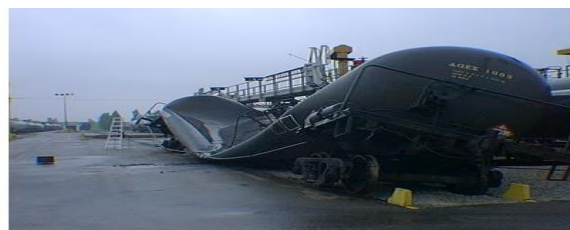
Figure: 2) Failure due to external pressure
