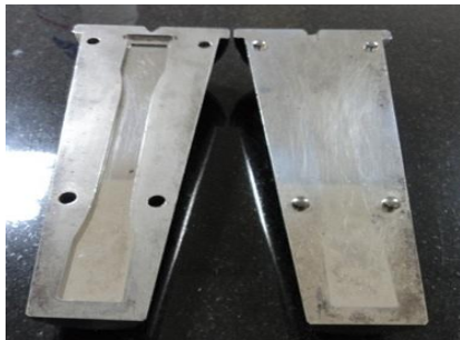
Fig: Tensile test specimen dies as per ASTM D638
