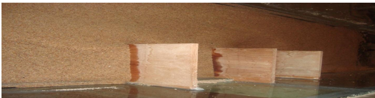
Plate (1): Front view of the groynes
