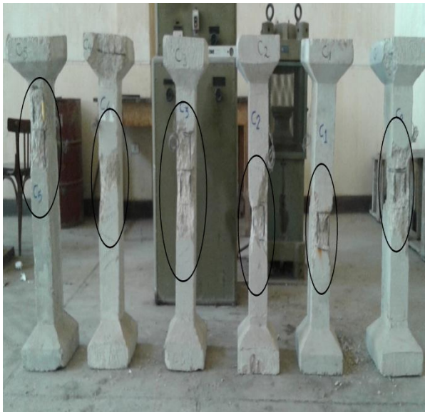
Figure 3 Specimens after testing before retrofitting.
