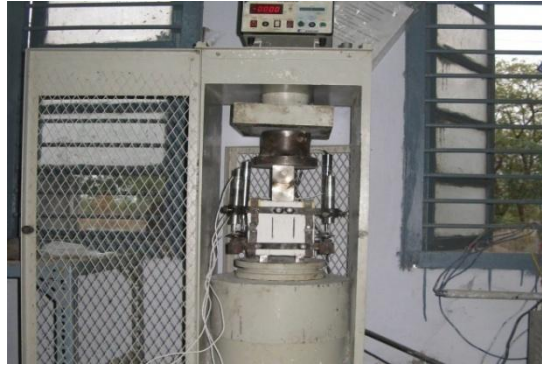
Plate 4. Test setup for DCN specimen
