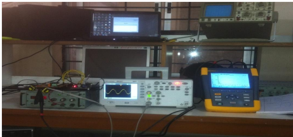
Fig: 11 Experimental setup of H6 inverter circuit for measurement of harmonics
