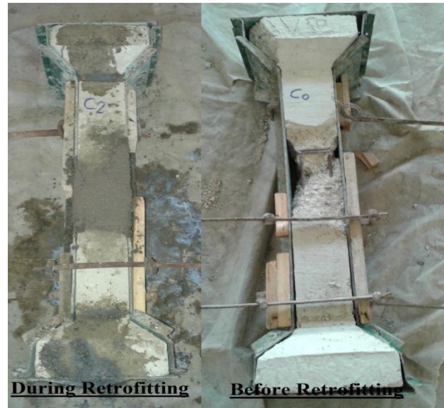
Figure 4 Details of retrofitting columns with Grout mortar.
