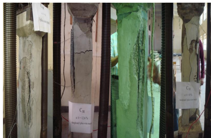
Figure 14: Failure Modes of Strengthened Columns
