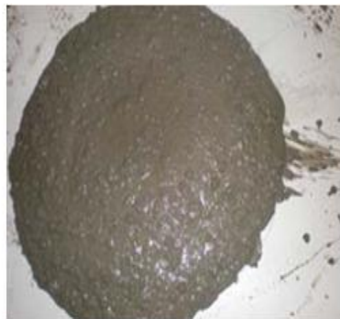
Fig3.4 Selfconsolidating concrete using metakaolin
