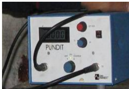
Figure 3: Portable Ultrasound Non destructive Digital Indicator Tester Equipment (PUNDIT)
