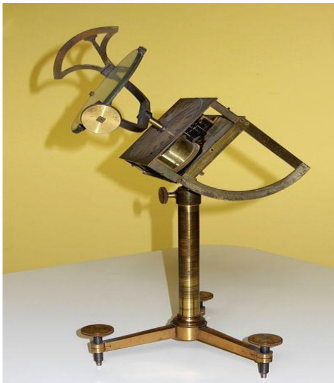
Fig.3 Heliostat Device for Solar power collector
