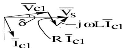
Figure(3) : phasor diagram for reactive power flow to the DSTATCOM
