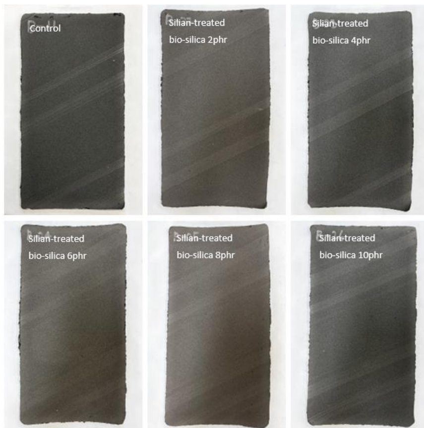
Figure 6. Variation in the internal foam structure of EVA foams depending on silane-treated bio-silica content
