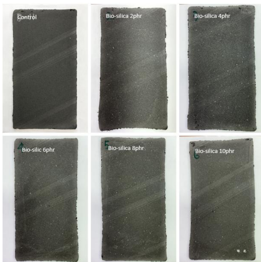
Figure 5. Variation in the internal foam structure of EVA foams depending on bio-silica content
