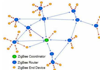
Figure 1-Typical ZigBee WSN – Mesh Architecture
