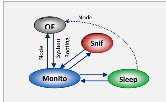
Figure 3 – Sensor Node State Transition
