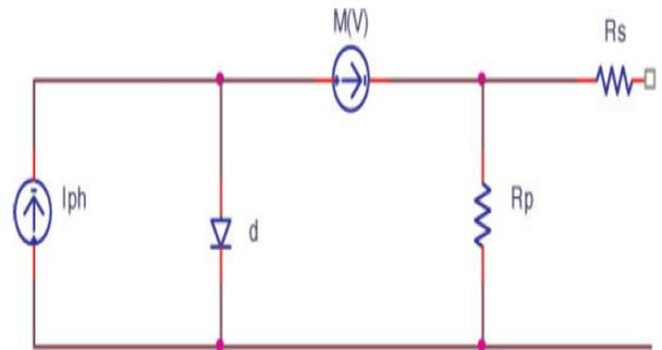
Figure 1: Solar cell equivalent circuit considering the avalanche effect
