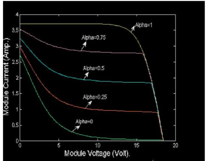
Figure 8 :I-V characteristics of the photovoltaic cell under shadow
