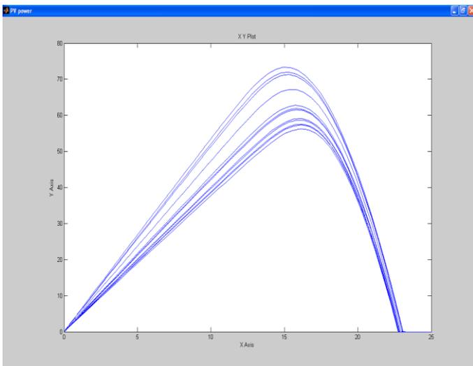
Figure 6 :P-V characteristics of the photovoltaic cell under different isolation
