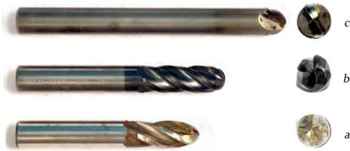
Figure 1.a) HSS Ball Nose, b) Carbide Ball Nose, c) PCD Ball Nose
