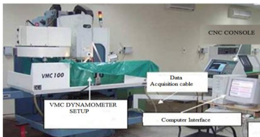
Figure 2. Experiment setup with dynamometer arrangement
