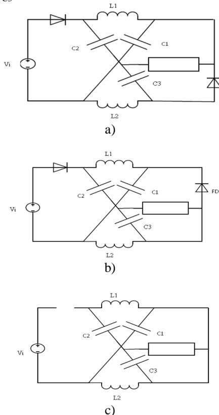
Fig.4. Equivalent circuits of MZS single-phase inverter for (a) State 1 (b) state 2 (c) state 3.
