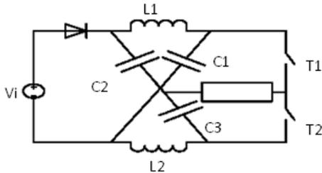
Fig. 3 .MZS single-phase inverter with two switches.
