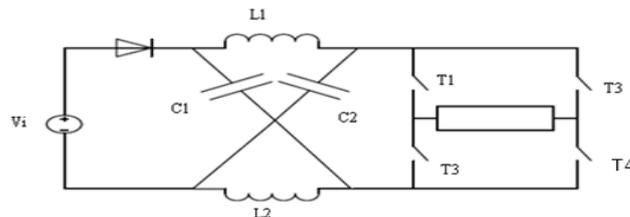
Fig.1. Z-source network with 4 switch single-phase inverter.
