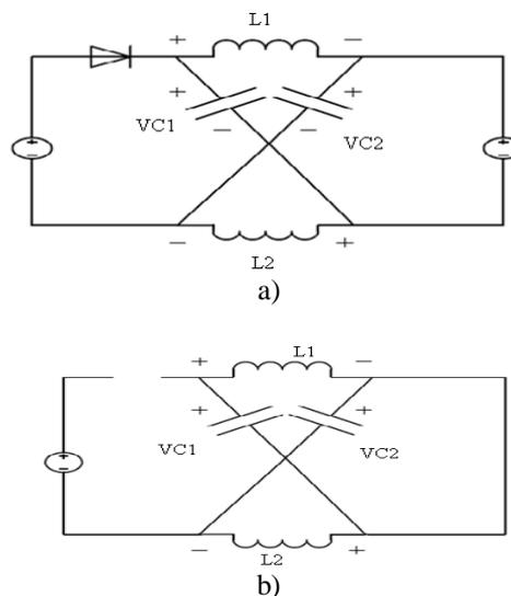
Fig.2. Equivalent schemes of the Z-source network in (a) non-shoot through state (b) shoot-through mode
